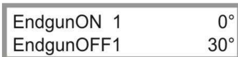
Fig. 4.6 Parameters for setting of ON and OFF range of endgun
