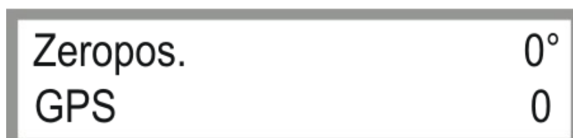
Fig. 5.15: Parameter for shifting of zero position and for GPS activation
