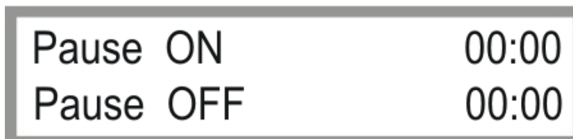
Fig. 4.10 Parameter for setting start and stop time for irrigation pause
