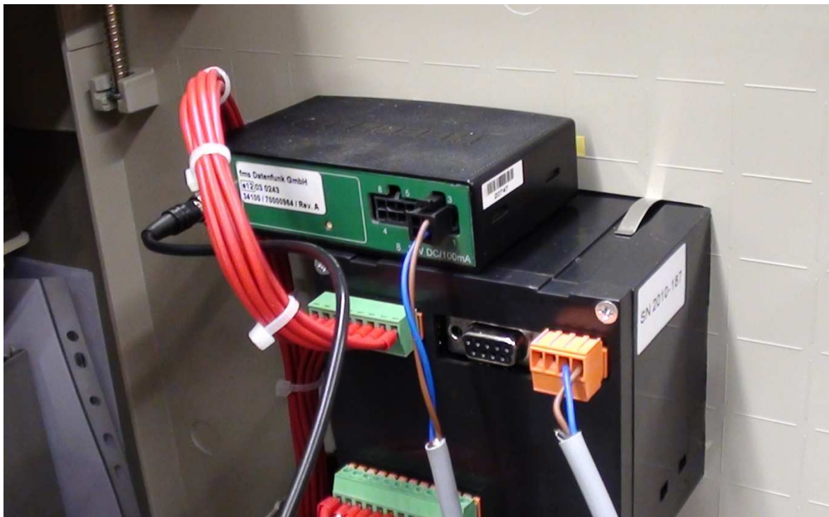
Fig. 2.1: Connection of GPS module with Pro module
