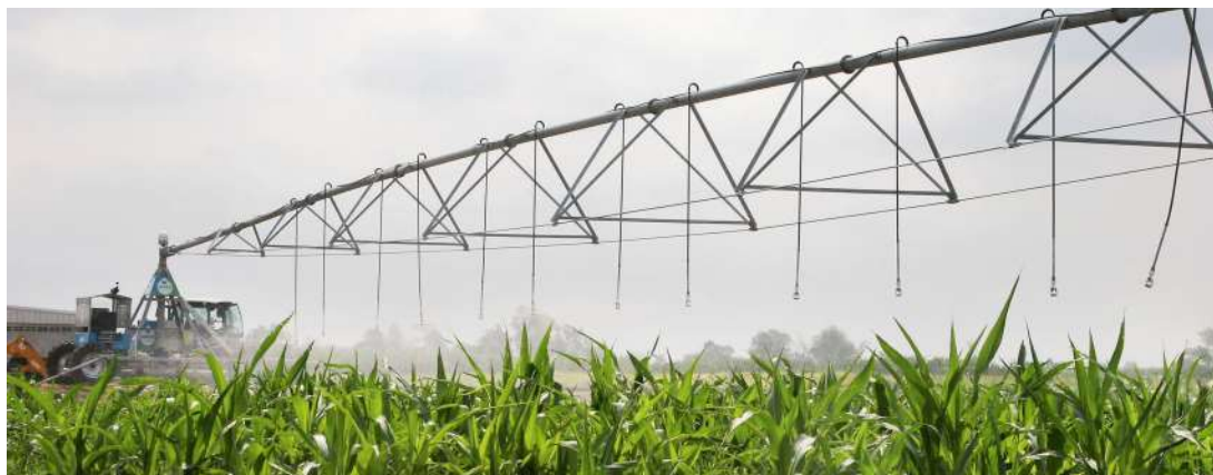
The Centerliner with a system length of 330 meters irrigates 88 hectares.
